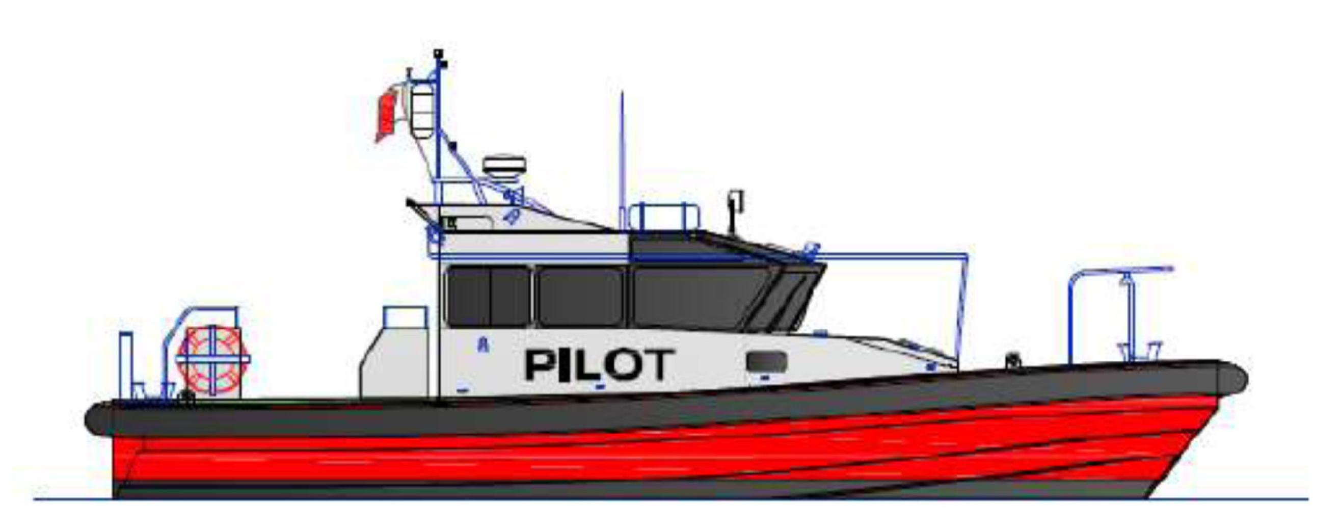
This Pilot Boat is one of a series of Fast Pilot Boat designs by Camarc. The double chine hull gives exceptional all-round seakeeping and has been proven on over 100 pilot boat craft in service worldwide.
